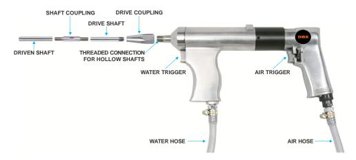
**Operation:** The portable pneumatic tube cleaners use hollow shafting of different diameters as per tube I.D. to be cleaned which can be coupled together to form lengths as per the length of the tube to be cleaned.
