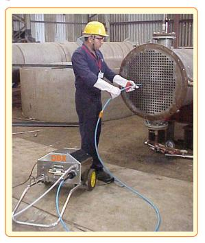
DBX Model ATC-300 Extra Heavy Duty Pneumatic Tube Cleaning Machine includes air filter, regulator, lubricator, adjustable speed/torque control, mobile dolly, tool storage box and air foot padel.
